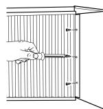
4. While the right-hand curtain is still extended, insert #10 x ¼" pan-head Phillips screws into the top and bottom slots of curtain. Screw curtain to the top and bottom holes in air conditioner cabinet.
